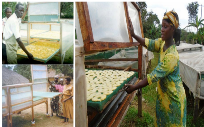
Fig. 1: Solar dryers made from local materials in Uganda. (a) mango drying and (b) pineapple drying
