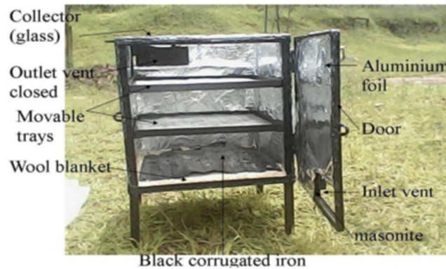
Fig. 3: A constructed convectional solar dryer
