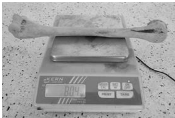
Fig. 1: Measurement of humeral weight using a digital (KERN 440-45N) machine
